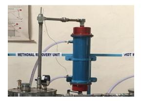
Sheet and tube (copper tube). Shell side (Water Flow) Tube Side (Methanol flows Copper tube inner dia: 12mm Copper tube dia: 14mm Total copper tube: 6 no's Over all diamantine: 300mm height \*120mm dia
