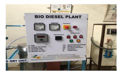
All temperature sensors, 3 Heater coil, pump switch, two stirrer motors, switches, along with voltmeter, and analog meter, Main tank temperature controlling unit are provided in the electrical panel bord
