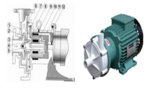
These pumps are 100% Leak Proof Magnetic Drive pumps. There is no shaft seal used and the impeller provides the rotation with the help of Magnetic drive. High Power permanent rare earth Magnets are used in magnetic drive arrangement which gives high mechanical efficiency with zero slippage.
